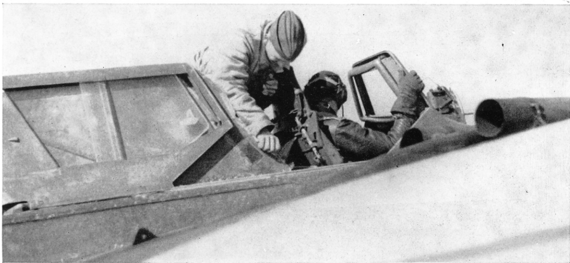
A Henschel pilot prepares for a sortie in Russia. Note the massive construction of the cockpit, a self-contained unit composed almost entirely of armour plate.
