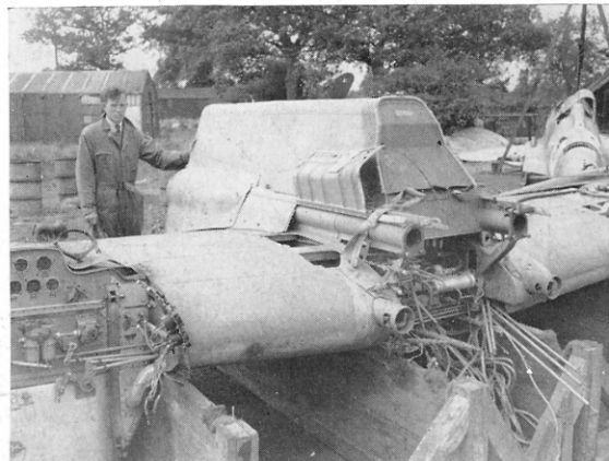
Another view of the dismantled Henschel shows the blast tubes for the nose guns, and the massive strength of the centre-section. (Photo: P. E. Castle)
