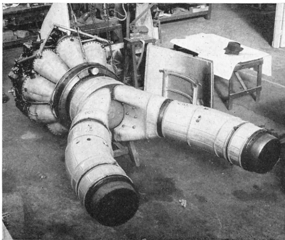
The Rolls-Royce Nene engine with Hawker's patented bifurcated jet pipe. (Photo: F. K. Mason collection)
