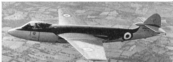
Introduced during the initial production run at Hawkers was the bullet fairing on the tailplane seen here on WF159.
