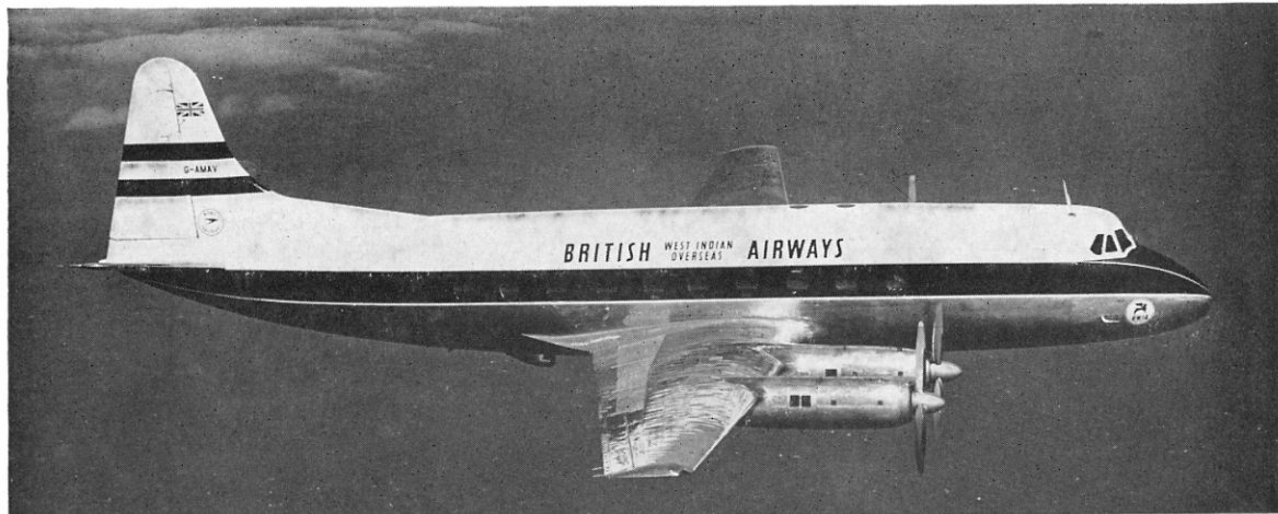
G-AMAV, the Type 700 demonstrator, in the livery of British West Indian Airways. Note the ventral air conditioning intake which appeared on early Viscounts.
