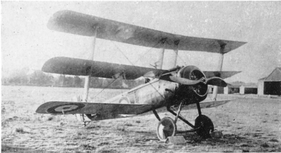
Apparently one of the six triplanes built by Clayton and Shuttleworth with twin Vickers guns. (Photo: Imperial War Museum Q60483)
