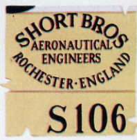
Manufacturer's plate displayed both sides of rudder (port shown) of S.106 illustrated above.
