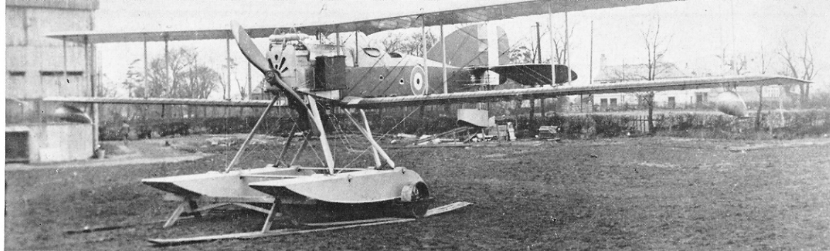
Sage-built Short Improved 184 powered by the 240-h.p. Renault engine with the original installation that embodied two flank-mounted radiators. This aircraft also has the later type of wing-tip floats.
