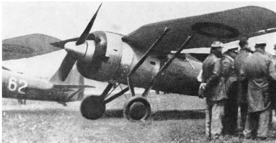
Roumanian P-11b's, powered by the K.9 engine. Note early Roumanian Air Force roundel markings under wing-tips. (Photo: via the author)
