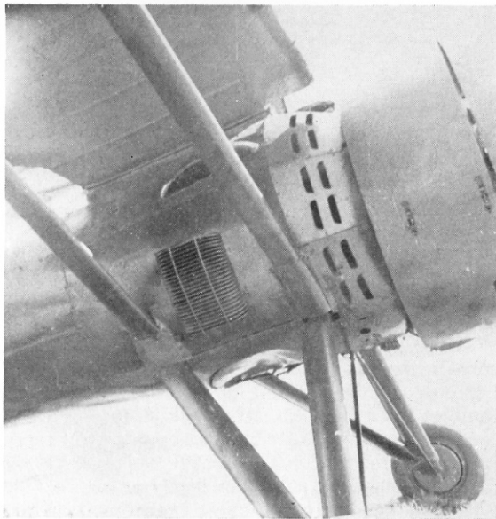
Details of the P-11c: (above) Cowling (note jettisonable fuel tank visible on underside of fuselage); (right) Main undercarriage gear. Photos: via the author.
