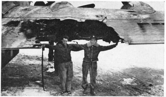
Battle damage 1: this Fortress returned to base safely after a burning wing tank had destroyed 30% of the wing root. (Photo: W. J. Connell collection)
