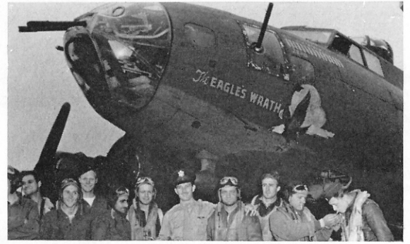
Left: "Sugar", a late model B-17F, displays the cheek positions usually associated with the B-17G. Right: "The Eagle's Wrath", a B-17F-20-BO, serial 41-24524, of the 91st B.G., with twin nose guns. The armour plate covering the bombardier's optical-flat panel is a pointed reminder of the B-17's vulnerability to head-on attack, one of the main reasons for the failure of the Unescorted Daylight Precision Bombing theory. (Photos: W. J. Connell collection)
