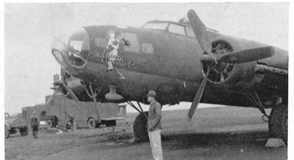
Left: "I Got Spurs", a B-17F-10-BO of the 3rd Recon. Group, 12th Air Force, based in North Africa; Group Commander was Col. Elliot Roosevelt. Note "dimple" nose transparency and Tri-Metrogon window under nose. (Photo: U.S.A.F.). Right: The famous "Piccadilly Commando"; note lack of guns in nose transparency. (Photo: W. J. Connell collection)
