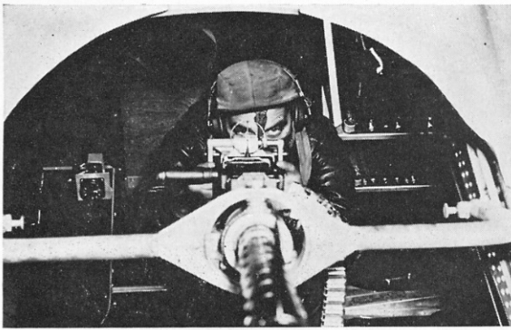
Messerschmitt's eye-view of a B-17F radio-operator's .50 cal. gun in the O-type mounting. (Photo: W. J. Connell collection)
