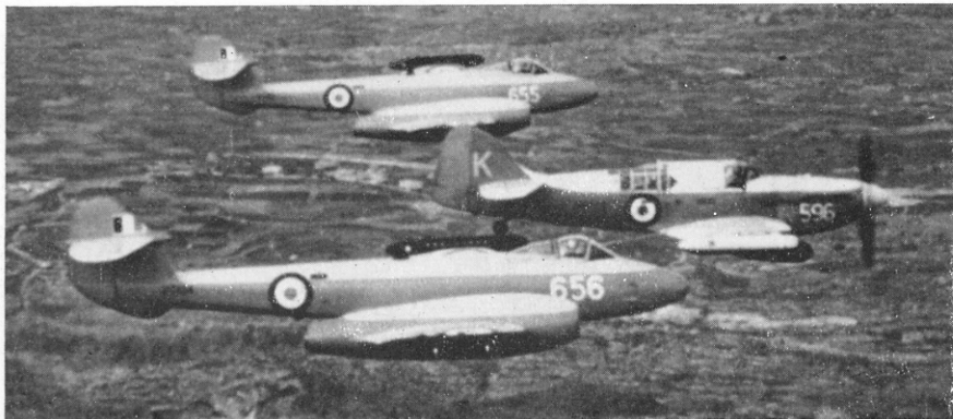
At the end of a long career, albeit not exciting, a large number of Mk. 4s were converted to drones. As such they were designated the Meteor U Mk. 15. Illustration shows two manned U.15s under the control of a Firefly drone over Malta.
