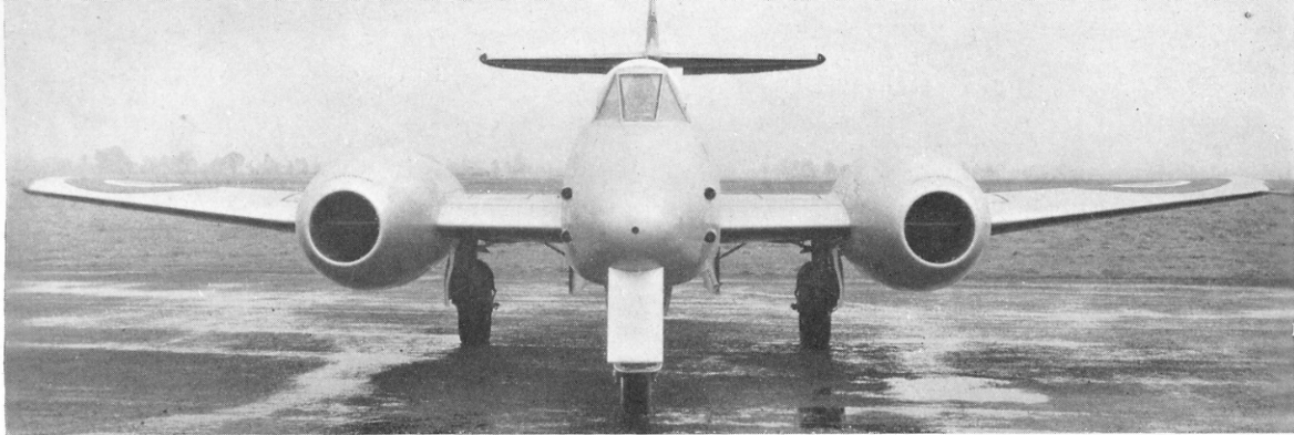
The small frontal area and clean lines of the Mk. 4 show up well in this head-on view. It also illustrates the good grouping and positioning of the four 20-mm. guns and shows the cine camera vision tube in the nose.
