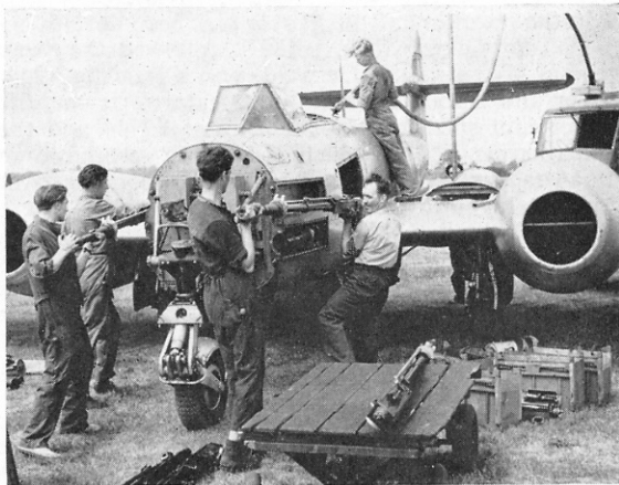
In the field with the Meteor 4. Above: high-speed refuelling of a Norwegian Mk. 4. Below: armourers change the four 20-mm. cannon. (Photos: Ministry of Defence)
