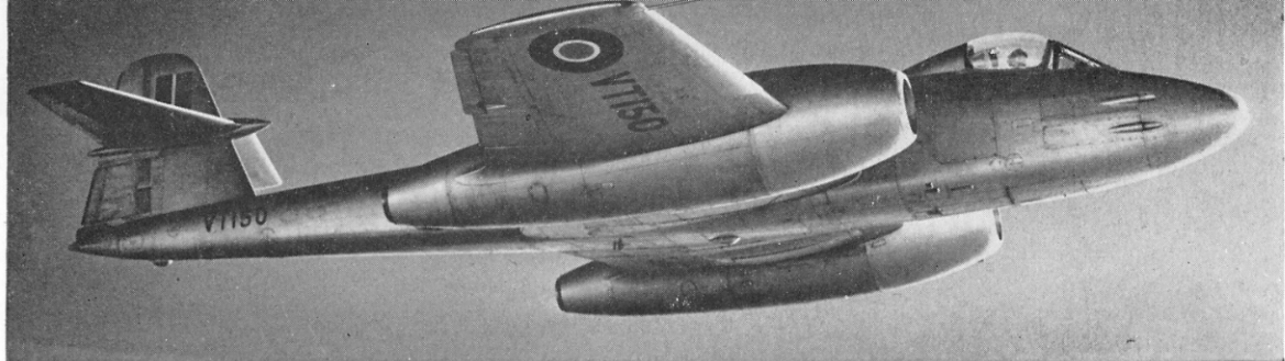
The prototype Meteor F. Mk. 8 was VT150, originally produced as an F. Mk. 4. Modification of the Mk. 4 airframe included a new tail assembly and a 30-inch fuselage extension. (Photo: Hawker Siddeley Aviation Ltd.)
