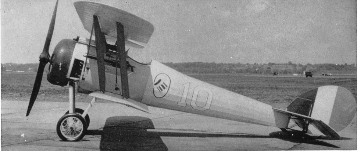
Restored Nieuport 28 with standard wings and struts owned and flown by Cole Palen of Old Rhinebeck, New York. Markings are authentic, but machine is not camouflaged. Note how far propeller hub projects ahead of shallow-chord Thomas-Morse cowling. (Photo: E. M. Sommerich collection)
