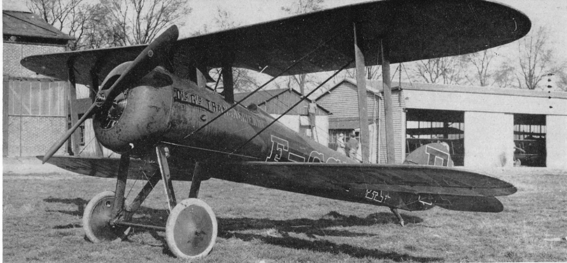
A post-war civilian conversion with an 80-h.p. Le Rhône engine. Although carrying French registration, this must have been an A.E.F. left-over because the "Lift Here" placards on the fuselage are in English. (Photo: SAFARA)
