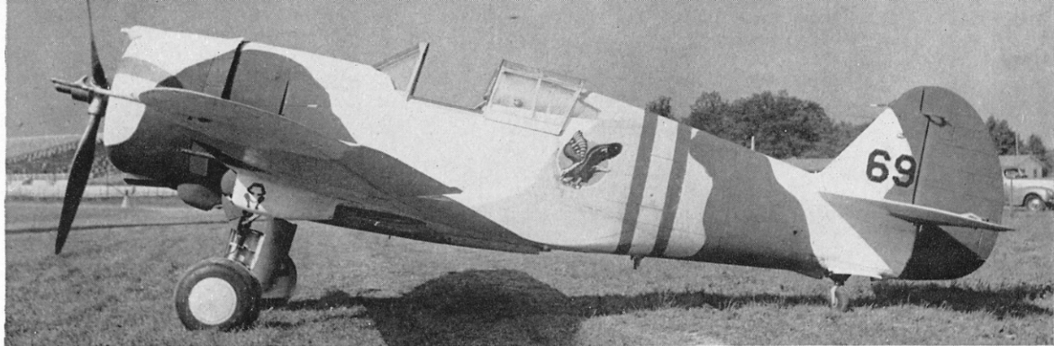
Above: A P-36C, probably of the 27th Pursuit Squadron, with the experimental camouflage of the 1939 War Games. The external underwing ammunition box for the .30 calibre wing guns is clearly visible. (Photo: courtesy Gordon S. Williams.) Below: Another P-36C with a different War Games camouflage pattern; these schemes were applied with washable paint and could easily be removed. (Photo: courtesy William T. Larkins)
