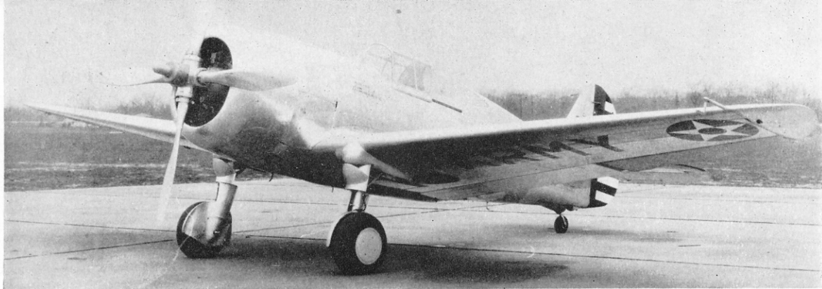
Curtiss Model 75E, one of three tested by the Air Corps as Y1P-36. The machine illustrated, serial 37-68, has been fitted with an experimental four-blade Curtiss electric propeller. (Photo: U.S.A.F.)
