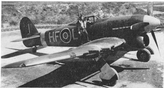
For many months No. 183 (Fighter) Squadron flew Typhoons on fighter-bomber strikes. These two pictures are interesting in that both aircraft are carrying the same code letters; that above, R8884, was one of the first Typhoons modified to carry underwing bombs (note old canopy and unfaired cannon). JR128 displays faired exhaust stacks, faired cannon, sliding canopy, whip aerial and 3-blade propeller.
