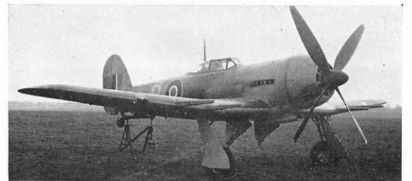
One of the interesting installations carried out on the Typhoon was that of the annular radiator with Sabre II and IV engines in R8694. By and large this was a successful experiment but disruption to production lines forestalled any interest by the Air Ministry. Top speed was quoted by Napier at 452 m.p.h.
