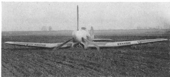
One of many Typhoon accidents, this Mark IA of No. 56 (Fighter) Squadron suffered engine failure and undershot the runway at Matlaske, Norfolk, in attempting a forced landing.
