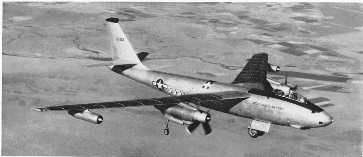
The first of two propeller-driven XB-47Ds on its first flight, August 1955. The XB-47Ds were B-47B airframes with Wright T-49 turbo-prop engines replacing each in-board pair of J-47 jets. (Photo: Boeing)
