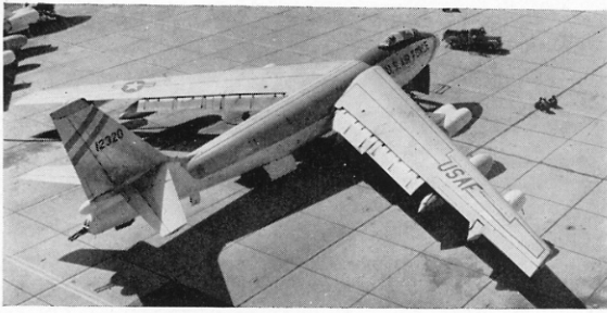
B-47B-II is B-47B modified to B-47E standard. Note how Fowler flaps increase wing area prior to assuming lowered position. (Photo: Gordon S. Williams)
