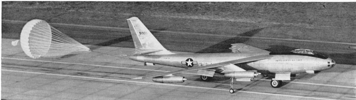
The No. 6 B-47A demonstrates the use of the thirty-two-foot diameter deceleration parachute.
