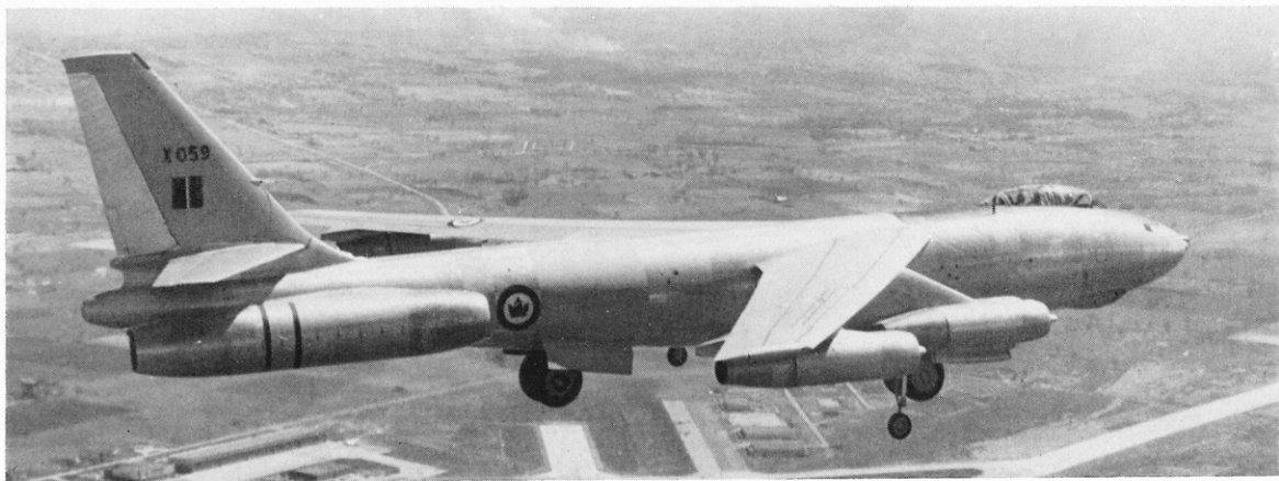
A B-47B loaned to Canada for testing of the Canadian-built Orenda "Iroquois" 20,000-lb. thrust jet engine. The airframe was modified by Canadair, Ltd., and designated CL-52. (Photo: Orenda)
