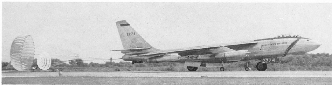
Lockheed-built B-47E-LM with both approach and decelerating parachutes still deployed near the end of the landing roll. (Photo: E. M. Sommerich)
