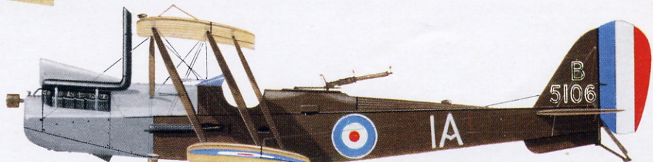
R.E.8, B5106 of No. 59 Sqdn. R.A.F., Vert Galand, May 1918. Fitted with deep sump cowling and navigation lights.
