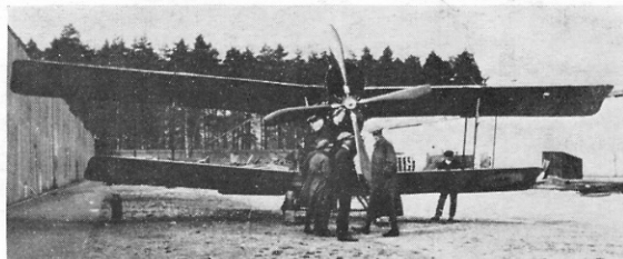
The R.E.8 B738 with supercharged R.A.F. 4d engine, R.A.F. variable-pitch airscrew and balanced rudder similar to that of A3406. The tall figure immediately to the right of the airscrew is Lt. Harold Elliott who was then in charge of the Engines Flight at Farnborough and flew as flight observer in this aircraft and in the Maori-powered R.E.9 A3561.
