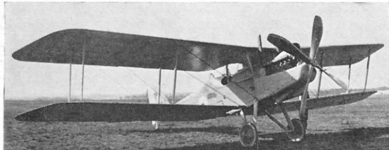
The third Siddeley-built R.T.1, with R.A.F. 4a engine, photographed at Farnborough on 30th October 1917. This photograph provides an interesting comparison with the R.E.9 A4600. (Photo: Crown copyright)
