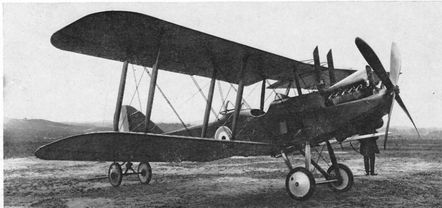
The R.E.9 A4600 at Farnborough, 24th September 1917, with enlarged upper fin. (Photo: Crown copyright)
