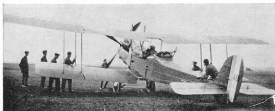
Left: The first production R.E.8, A66, photographed at Orfordness; no fixed gun is visible in this photograph. A66 later crashed at Orfordness and was quite extensively damaged. Right: A73 with Vickers gun installed inside the fuselage. The firing port and the connecting rod of the Vickers-Challenger interrupter gear can be seen. (Photo: Imperial War Museum Q55991)
