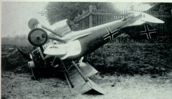
Confirmation of D IV's wayward characteristics when landing. D 3049/18 overturned by Lt. Speer. (Photo: Egon Krueger)
