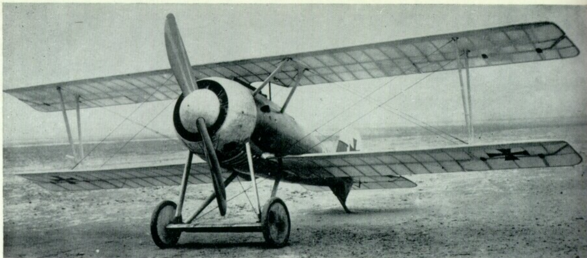
Further view of D 7551/17 after some modification to cowling. Note retention of "U" centre-section struts indicates modification not to full D III standard. First flew in this form 20th December 1917.
