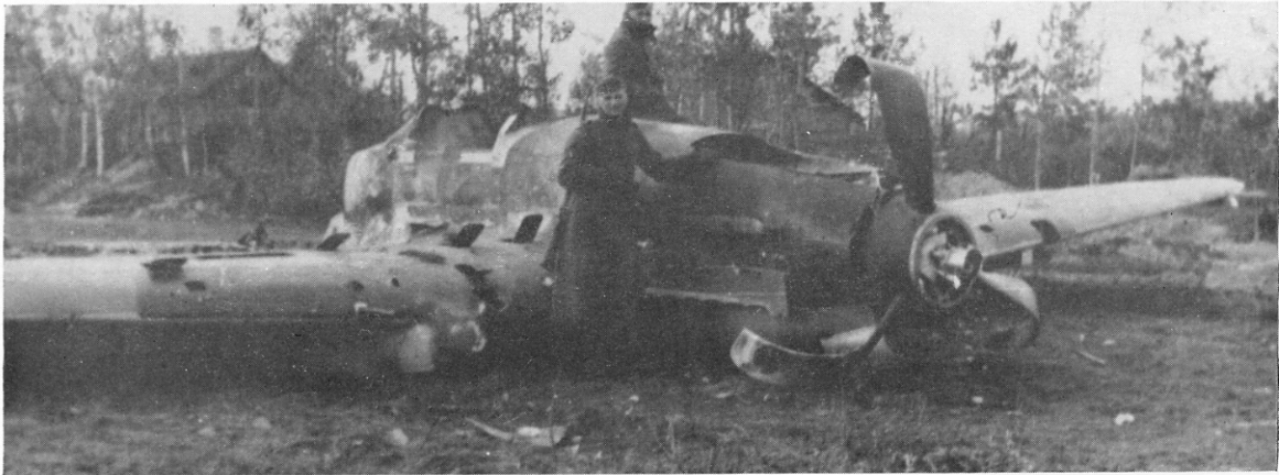
Below: Characteristically, this crashed Il-2 has broken in two behind the cockpit; the fuselage centre-section remains relatively undamaged despite severe punishment to the other sections of the aircraft.
