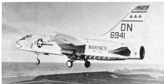
An F-8C, 146941, of VMF-33 during launching by steam catapult from U.S.S. Forrestal ; this photo was taken during the carrier qualification trials in the Atlantic.
