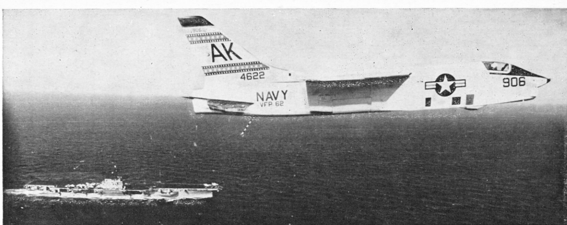
An RF-8A reconnaissance aircraft, No. 144622, of Navy Squadron VFP-62. The machine is seen here in the landing pattern over the U.S.S. Forrestal, with arrestor hook extended. (Photo: U.S. Navy)
