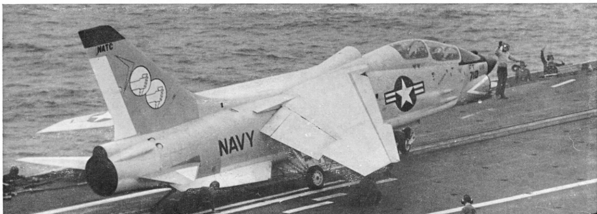
The sole two-seater Crusader trainer made ready for launching on the port catapult of the U.S.S. Independence. Note "Dual Control" fin emblem.
