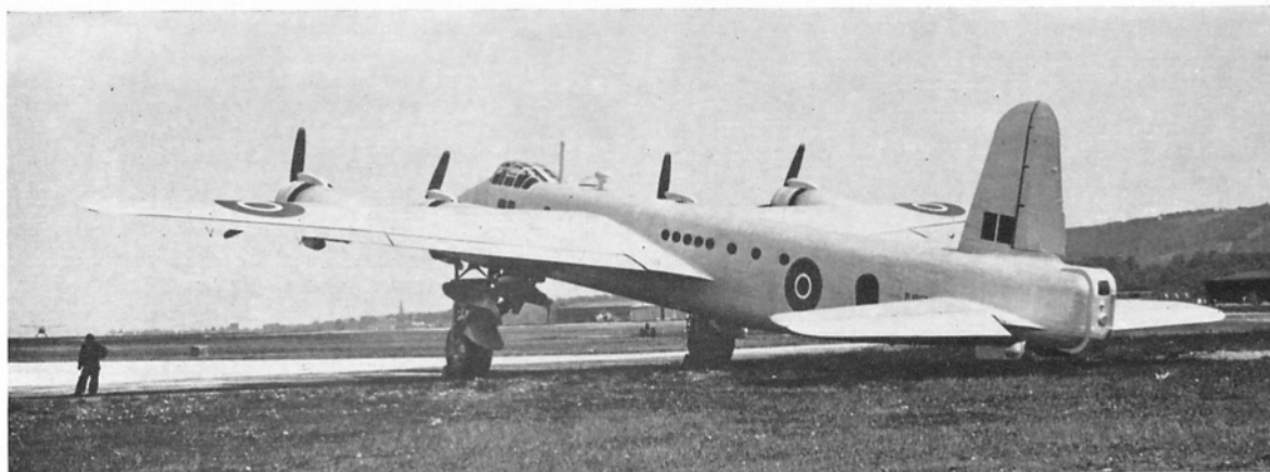
PJ958, the "Silver Stirling" converted to civil standards from a production Mk. V. Note faired-in tail turret.
