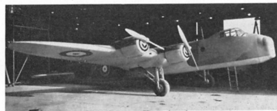
The half-scale wooden S.31 prototype in its pre-war colours. The S.31 in warpaint.
