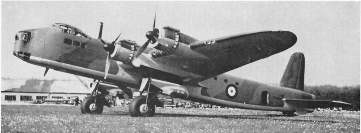
Second prototype Stirling L7605, with strengthened undercarriage.
