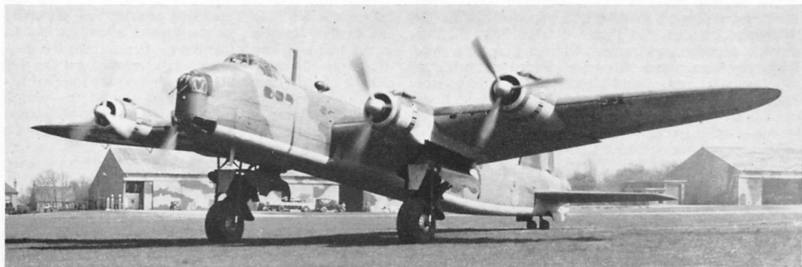
Second prototype Stirling L7605, with strengthened undercarriage.
