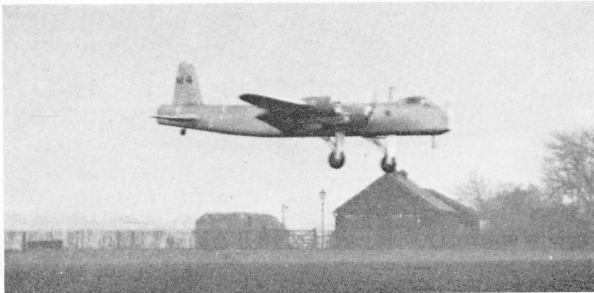
Rare flying view of the S.31. Powered by four 90 h.p. Pobjoy Niagaras, the "mini-Stirling" made its maiden flight on 19th September 1938, in great secrecy; the pilot was John Lankester Parker.
