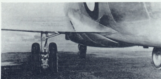
The twin-wheel "diabolo" gear of the "Barougan" and ventral "speedpack"—one of several wheel housings evaluated on these aircraft. (Photo: Messier)
