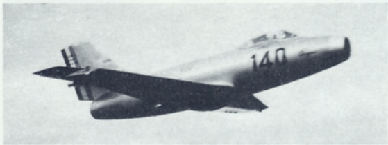
This picture of the first "Barougan" in flight illustrates an early type of main wheel fairing, into which the wheels retracted but were not enclosed. (Photo: via Cdt. Paul Boudier)
