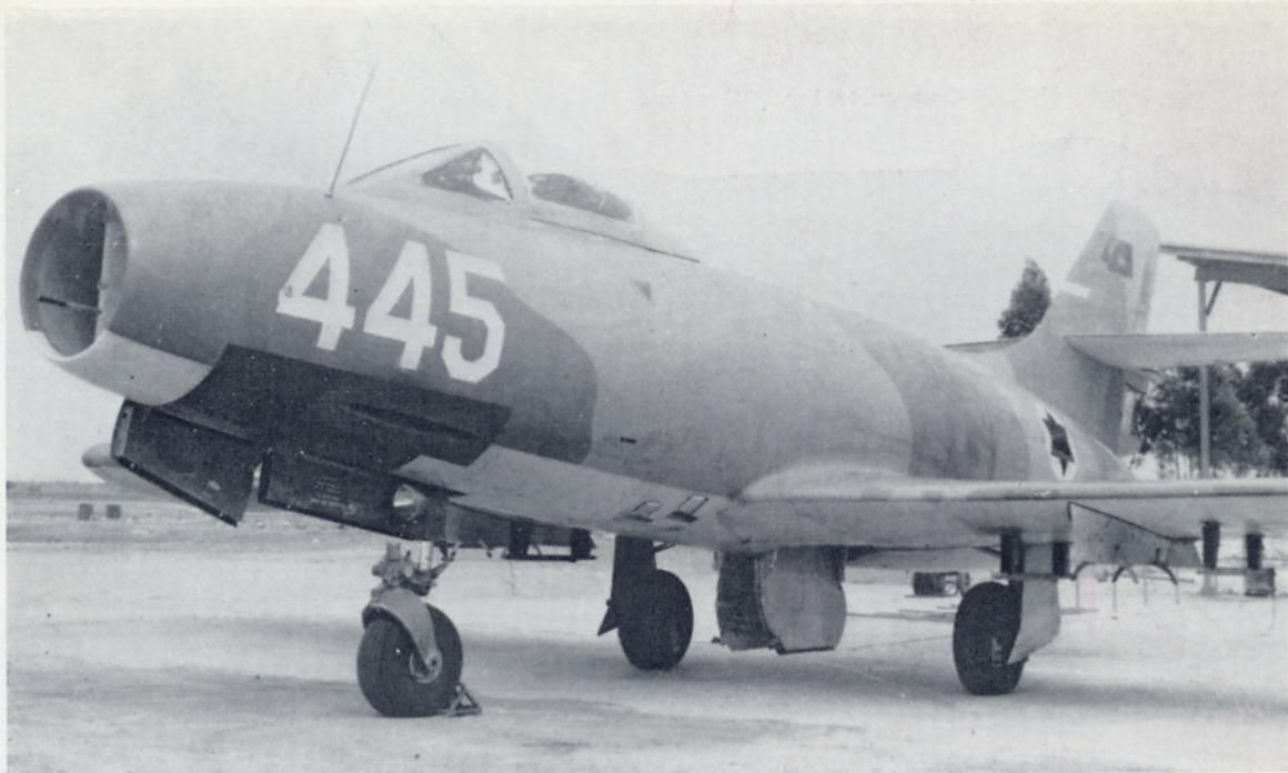
A more recent study of an IDF/AF Ouragan in desert camouflage of blue-grey and stone. Note the underwing attachment points for bombs and rockets. (Photo: Stephen P. Peltz)
