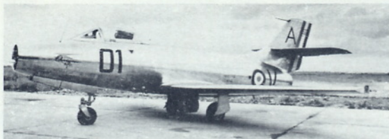
The first Atar testbed, M.D.450-10, proclaimed by the large "A" on the fin and nose serial "01". (Photo: SNÉCMA)
