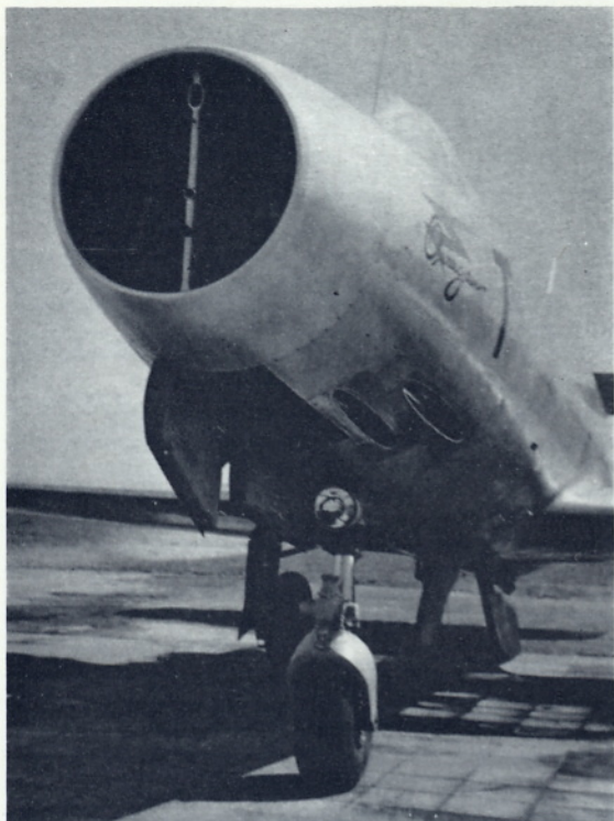
The redesigned two-piece nose wheel door fitted to all production Ouragans from No. 151 onwards. (Photo: Air-Britain via Charles W. Cain)
