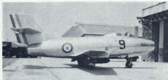
A previously unpublished photograph of the M.D.450-9 used to evaluate performance with various underwing loads. Note recording camera bulge immediately behind the nose wheel doors. (Photo: Cdt. Paul Boudier)
