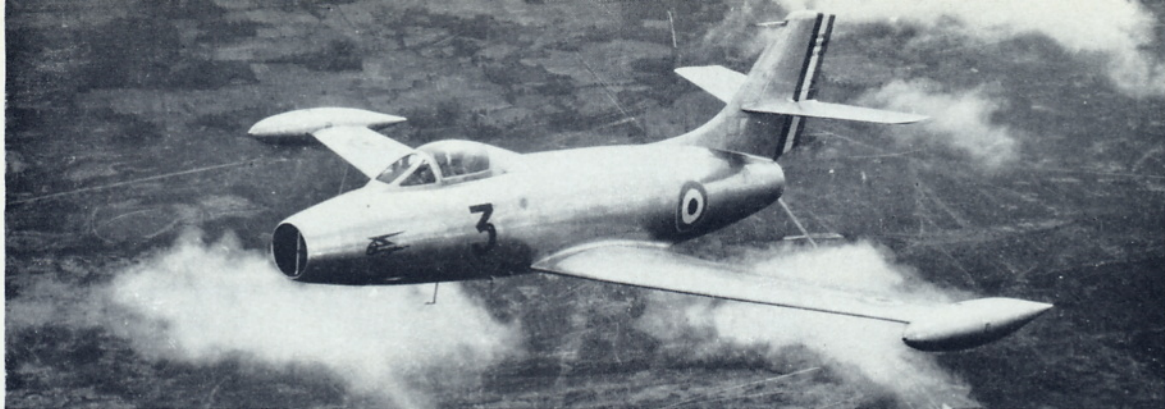
A fine aerial study of the third pre-series Ouragan: the tip-tanks still carry no fins. This aircraft was later the testbed for the HS403 afterburner developed for the Nene 104B. (Photo: Ministère des Armées "Air")
