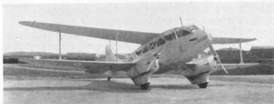
The military D.H.89, K4772, at Martlesham Heath on 26th April, 1935. Note extended dorsal fin, a Vickers Mk. V machine-gun and landing light in nose, five cabin windows (each side), navigation lights on wings and rudder, wooden propellers, and a deepened fuselage to house 4 x 20 lb. and 2 x 120 lb. G.P. bombs. Military Rapides were also sold to Spain, Iran and Lithuania.
