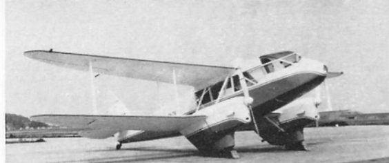
Owned by Avions Fairey S.A., OO-AFG (ex G-AKNV) was stripped down and completely rebuilt in 1958. Modifications included the installation of an electrical actuator (with indicator) for flap operation, 44 channels VHF radio, radio compass, a blue moulded perspex canopy over the pilot's cockpit and enlarged cabin windows. An extra folding door was fitted to allow the carriage of bulky cargo. The exterior was finished in red and white. (Photo: Avions Fairey S.A.)
