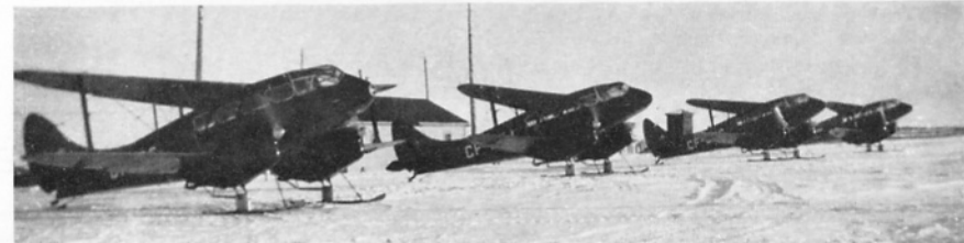
Four Rapides of Quebec Airways equipped with Elliott skis for the Rimouski to Harrington Harbour service during winter months. (D.H. Photo)
