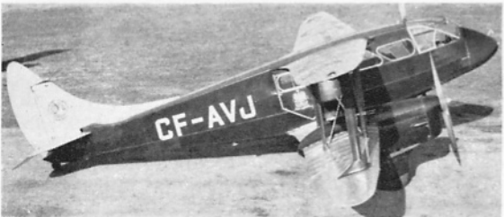
CF-AVJ, in full Canadian Airways livery and insignia, showing the additional starboard cabin door, was fitted with wheels for the Vancouver to Seattle service. This Rapide was destroyed by fire at Saint John, N.B. when the port engine exhaust started a fire during run up on 17th May 1939.
