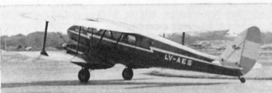
The Argentine Rapides present something of a mystery with regard to their origins, for ten were purchased shortly after the war by Sfredo & Paolini Ltd. for resale, while ZONDA are known to have had 15 Rapides at 28th October, 1948. LV-AES was one of six Rapides owned by Taxis Aereos Argentinos (TAASA) that had steel plated undersides to protect them from stones flung up on primitive airstrips. LV-AES, seen here at the Aeroparque, Buenos Aires, on 17th October, 1958, appears to be a Mk. 4. (Photo: F. A. Giró)
