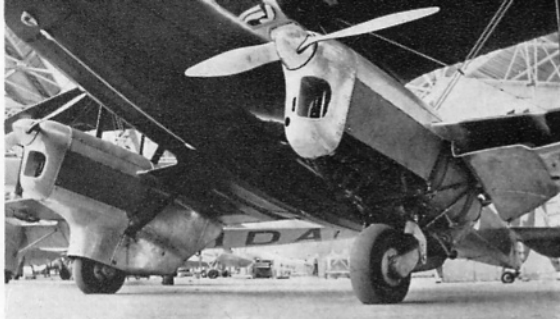
The Rapide E9, c/n 6420, experimentally fitted with a Dowty levered suspension undercarriage in 1938. (D.H. Photo)
