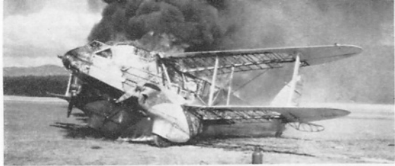
The sad sight of N.Z.N.A.C.'s ZK-ALC Tiora on fire at Rotarua airfield when exhaust flames from the starboard engine set the grass alight and subsequently itself. The burnt away fabric reveals the spars and girder wing structure. There were no human casualties. (Photo: N.Z. Herald)
