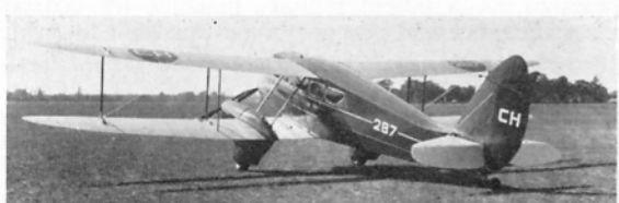
In May 1934 the prototype was sold to Herr R. Herzig of the Ostschweiz Aero Gesellschaft for service between St. Gaul, Zürich and Berne, in Switzerland. The fairing extensions and rudder balance flap had been removed by D.H.
