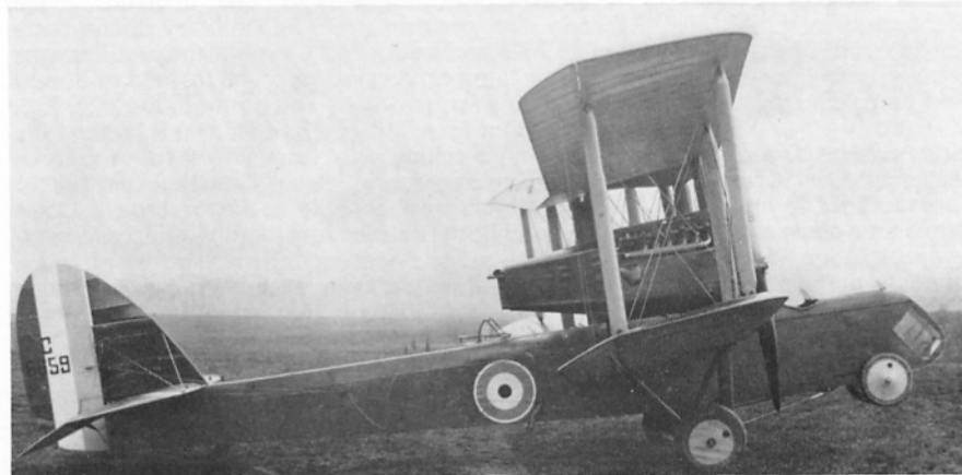
Left and above: The second prototype, C8659, with two Rolls-Royce Eagle tractor engines and transparent panels in the nose.
