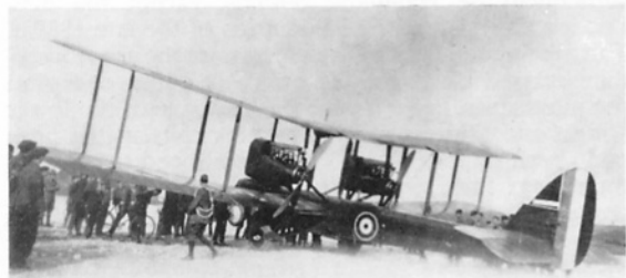
Above: The first prototype D.H.10, C8658, with two Siddeley Puma engines installed as pushers. When this aircraft was tested at Martlesham Heath Scarff ring mountings were fitted to the front and rear gunners' cockpits.
