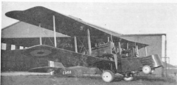
E5458, the D.H.10 that was modified for trials of the 1½-pdr. Coventry Ordnance Works quick-firing gun. It is here seen at Orfordness. The extended nose cockpit was plywood-covered, and nose wheels were fitted.
