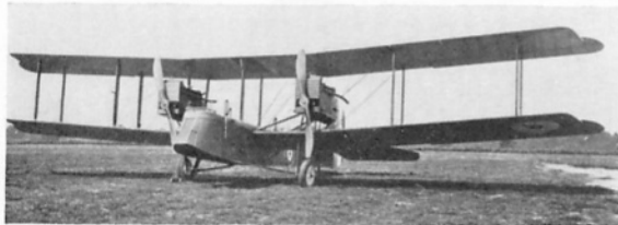
These photographs of the fourth prototype, C4283, were also made at Martlesham Heath, and provide an interesting comparison with those of C8660. These views show the reversion to slightly raked mainplane tips, the smaller and neater engine nacelles, the introduction of transparent panels in the nose, and the slight upward angle in the rear top decking of the fuselage owing to the increased angle of incidence of the tailplane. (Photos: Royal Aeronautical Society)
