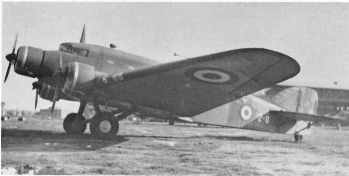
One of four S.M.81's acquired by Co-belligerent forces in Southern Italy after the armistice in September 1943; this aircraft has had the armament and wheel fairings removed. Note the streamlined radio aerial mast fairing and the D/F housing on top of the fuselage. (Photo: F. C. Dickey via R. Ward)
