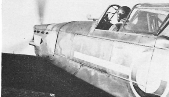
The hinged fuselage panels and turnover pylon are clearly shown in this view of a Vichy Air Force M.S. 406. (Photo: E.C.A.)
