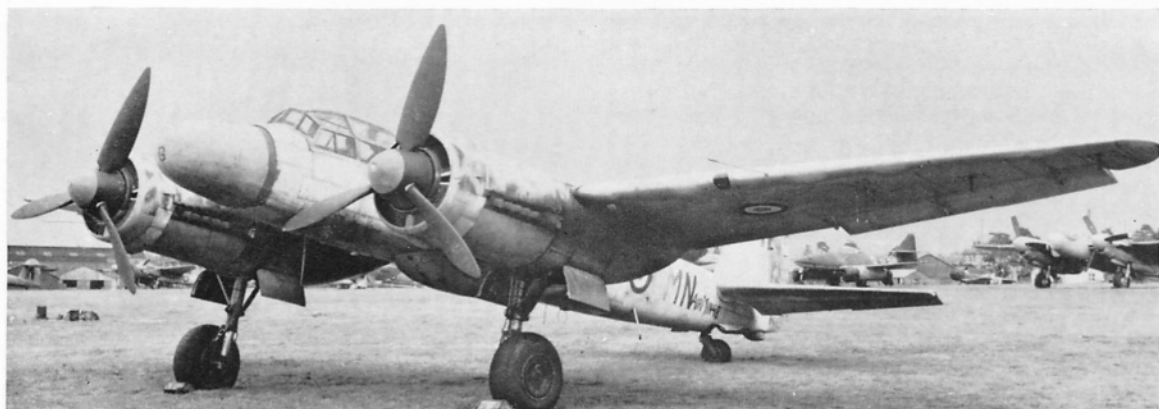
The final variant of the Ju 88 night fighter series, the G-7c. Ten examples were built before the German collapse; this aircraft carried the centimetric wavelength FuG 240 Berlin N-1a radar. (Photo: Imp. War Mus. MH4884)
