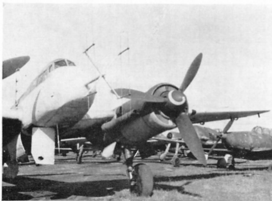
Ju 88G-7b fitted with FuG 218 Neptun radar and a Hirschgeweih aerial array. The elements were shorter than those used with SN-2, measuring only 90 cm. Note the belly entrance/escape hatch.
