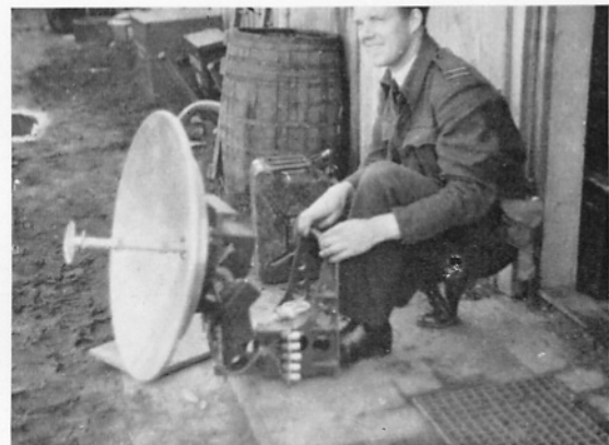
The aerial dish of the Berlin radar, which was housed behind the plywood nose cone of the G-7c.
