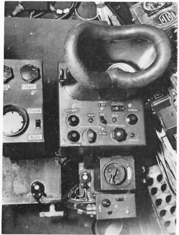
The radio operator's position, showing the indicators for the SN-2 radar (right) and the Naxos homing receiver (left). (Photo: Crown copyright)
