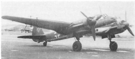
A Ju 88C-6b with Flensburg homing device and Lichtenstein BC radar. (Photo: Imp. War. Mus. HU2864)
