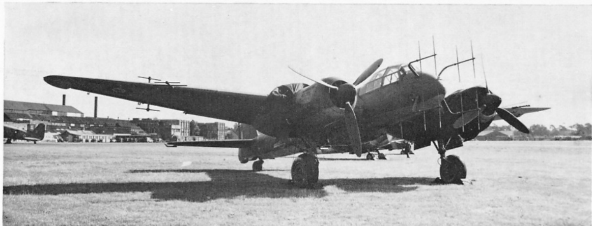
A view of 4R+UR at Farnborough; note Flensburg array on starboard wing.
