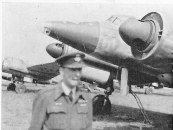
Another Ju 88G-7b with FuG 218 Neptun radar but fitted with the more streamlined Morgenstern aerial system. The aerial elements protruded through the plywood covering of the pointed nose cone.
