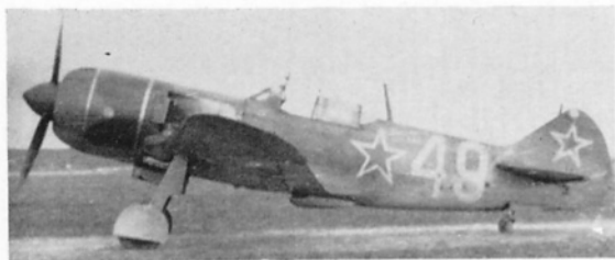
An La 7 of the 2nd Czechoslovak Fighter Regt. in 1945. Take-off power was increased by 200 h.p. over the La 5FN; and three cannons were sometimes fitted, two weapons being mounted asymmetrically to port of the centre-line. (Photo: the author)
