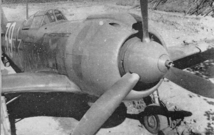
Nose details of the La 5FN, the most widely used of the wartime Lavochkin fighters. "FN" indicates Forsirovannyi Nyeoposredstvenno—"Direct boost", in reference to the direct fuel injection of the M-82FN powerplant.
