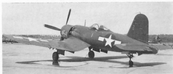
Another view of F2G-1 BuNo 88454, showing exhaust details. (Photo: Goodyear)
