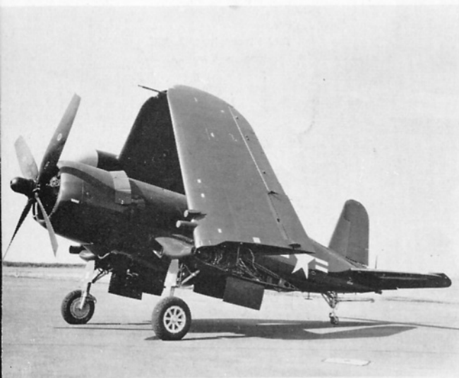
F4U-5N with wings folded; the small "bucket" on the starboard leading edge close to the fold line protects the gun camera from muzzle flashes during night combat.
