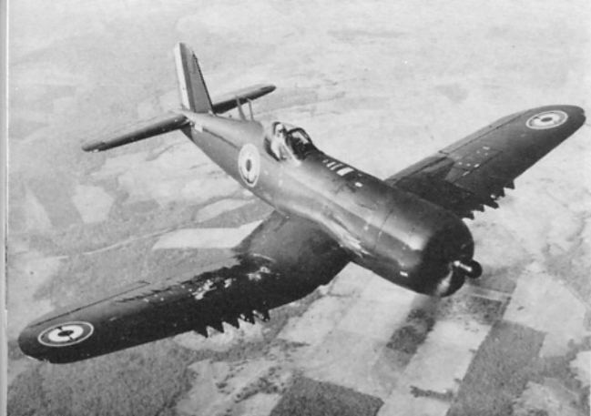
F4U-7 for the French Aéronavale during a flight test in the U.S.A. The fuselage lines of the F4U-5 were retained; in common with the -5 and AU-1 there was a widening ahead of Station 91 \frac{1}{2} .
