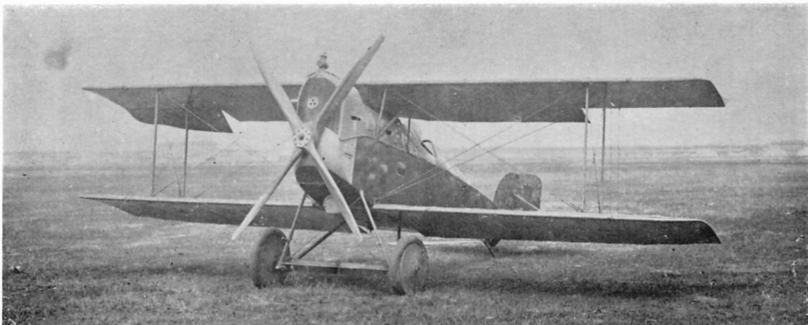
The four-blade Jaray airscrew, with inconsistently-angled blades, was fitted to 138.105.
