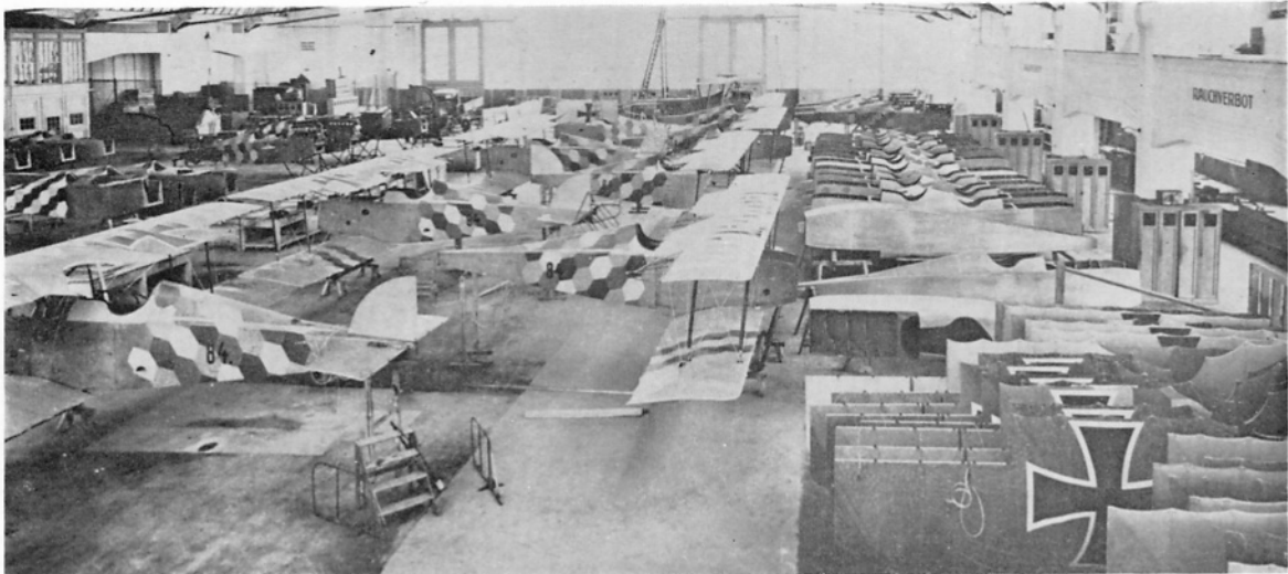
The W.K.F. workshop, showing production of Berg D I series 84 machines. Note the inboard position of the national markings on the stacked wings. (Photo: Peter M. Grosz)
