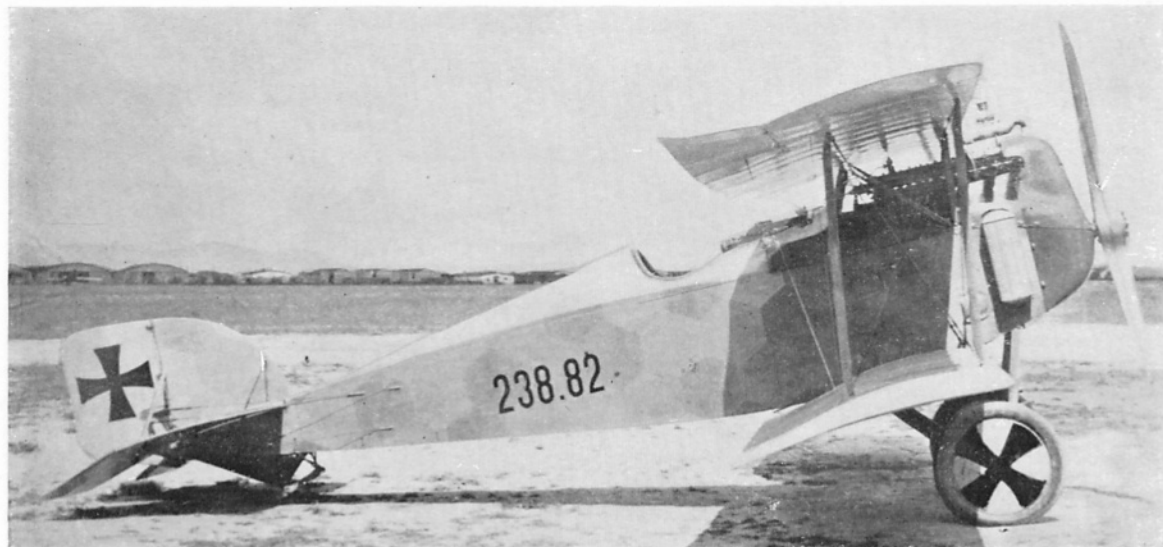
238.82, an aircraft of the third Aviatik batch; one of the few aircraft fitted with side radiators.
