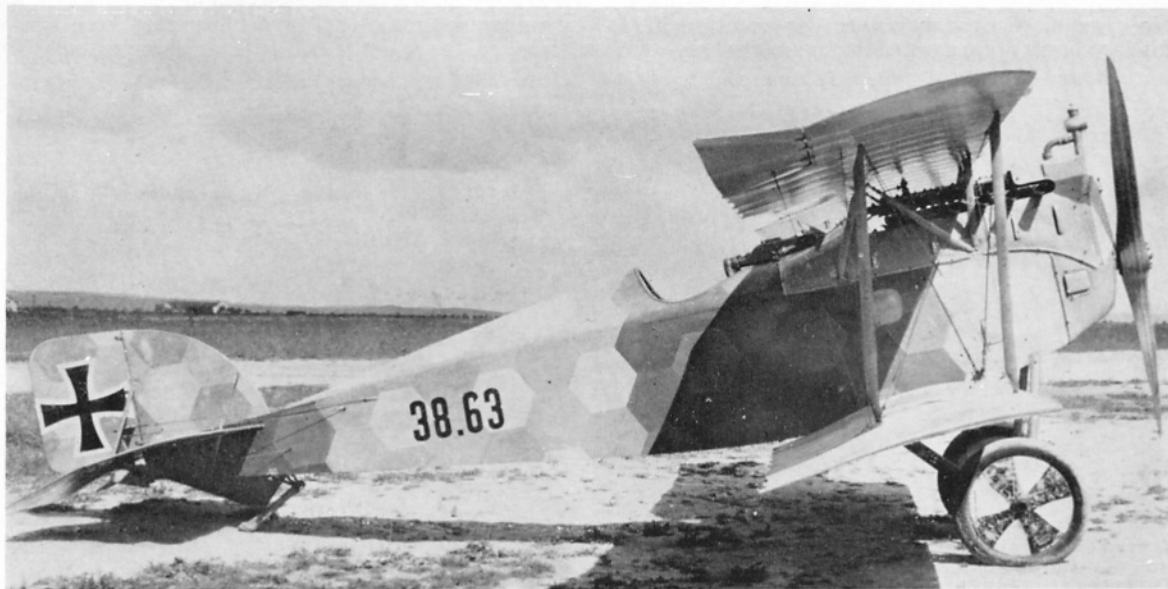
A fine study of No. 38.63, one of the first Berg D I's fitted with machine-guns immediately ahead of the cockpit, with breaches accessible to the pilot. Note darker-coloured hexagons painted in the cockpit area.
