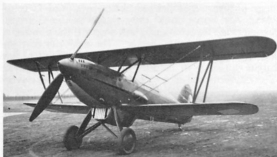
(Top left & right) The Avia B-534 in the first, second, (middle left & right) third and fourth production series configurations; (bottom left) the Bk-534, with a third 7.7 mm. gun between the cylinder banks; and (right) the B-634 of 1936 with cantilever undercarriage. (Photos: Avia)
