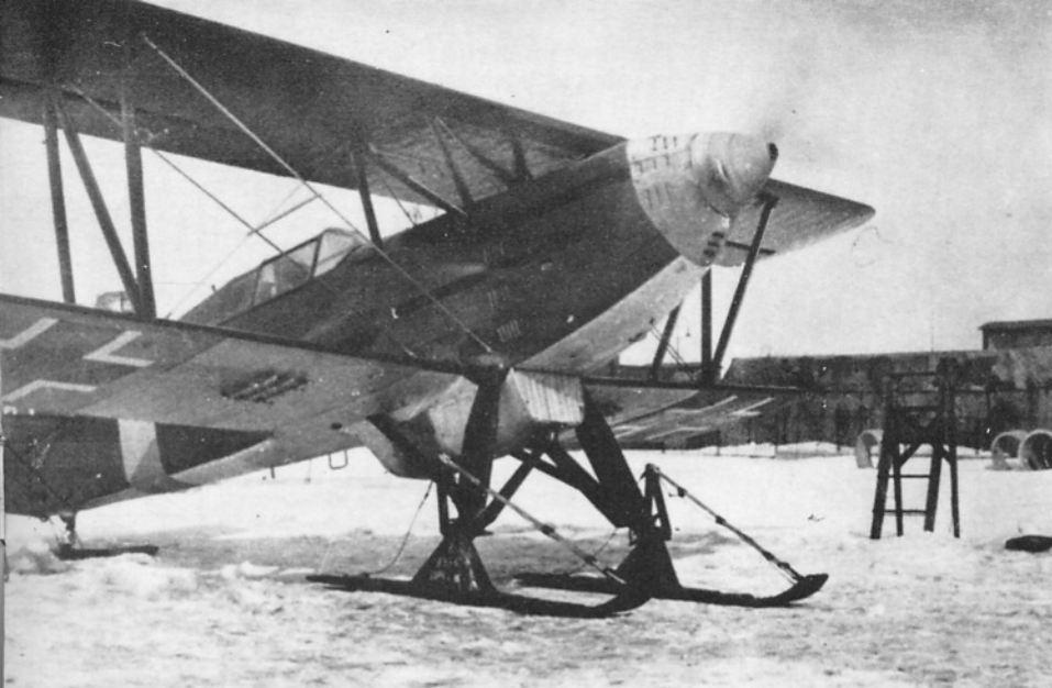
A ski-undersurface Bk-534 at Trenčin before delivery to the Slovak Air Force elements in Russia during the winter of 1941. Note olive-painted undersurface of top wing, and German-style markings on yellow tips of the lower wing. (Photo: Ing. S. Androvic)
