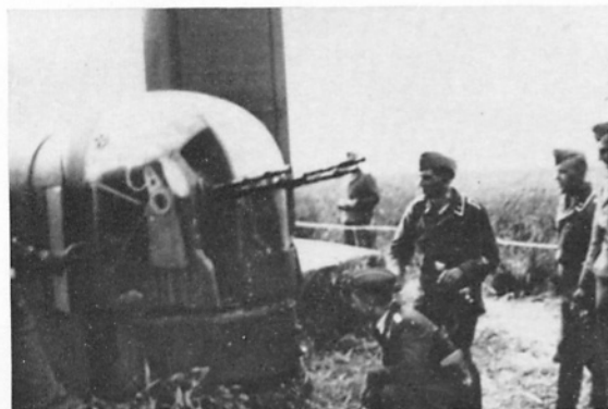
Luftwaffe "flak" personnel examine the Nash and Thompson tail turret of 102 Squadron Whitley V N1377 which crashed at Spijkenisse, Holland, on 31st August, 1940.
