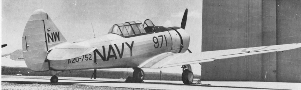
Wirraway III A20-752 was originally a CA-16 but was later converted by Commonwealth to a CA-20 (see p. 10) and used at the Royal Australian Naval Air Station, Nowra. (Photo: P. Ricketts)
