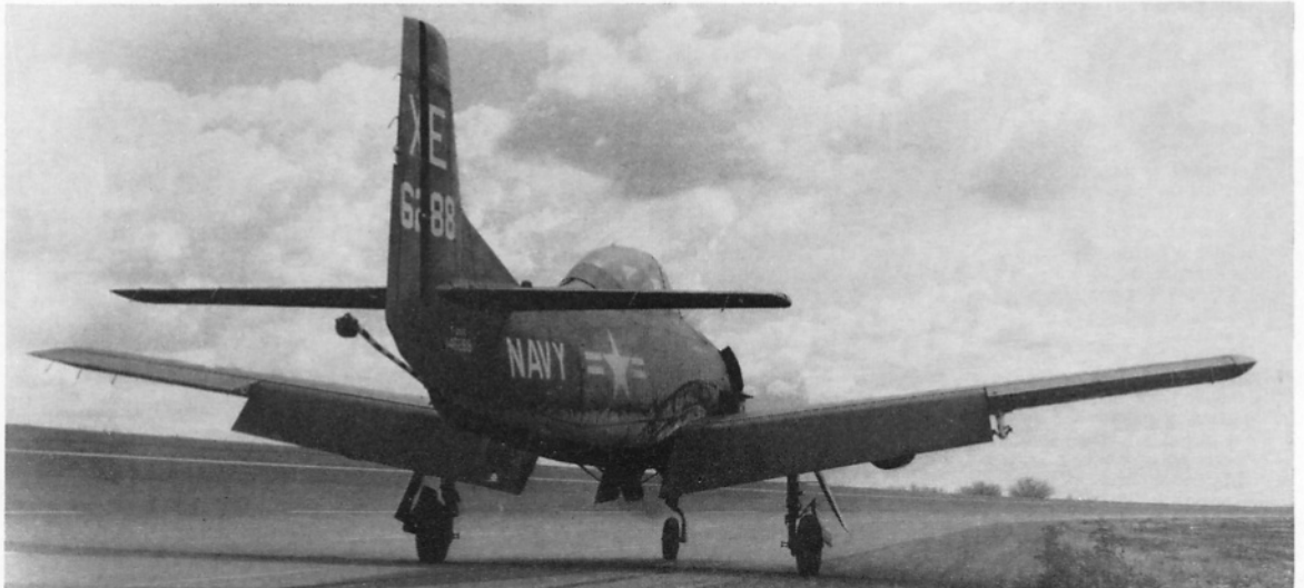
A T-28C during circular runway evaluation tests at General Motors' Mesa, Arizona, test track. Visible just below the open cowling flap is the spin recovery strip installed on T-28C's when underwing stores are carried. (Photo: U.S.N. via Naval Aviation News)
