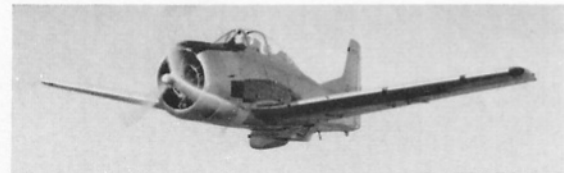
A reconnaissance version of the T-28D carries three cameras in a protruding pack under the belly. (Photo: N.A.A.)
