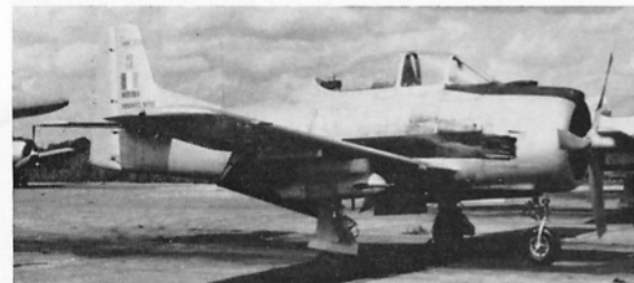
France purchased 245 T-28A's, which were subsequently put through an extensive modification programme by Sud Aviation. Re-engined, armoured, and with considerable underwing stores capability, the result was the ground-attack aircraft known to the French as the "Fennek" (Photo: Stephen Peltz via R. Ward)
