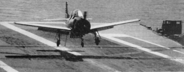
An interesting sequence showing a U.S. Navy T-28C performing "touch and go" on the U.S.S. Lexington. Note extended speed brake in landing view. (Photos: the author)
