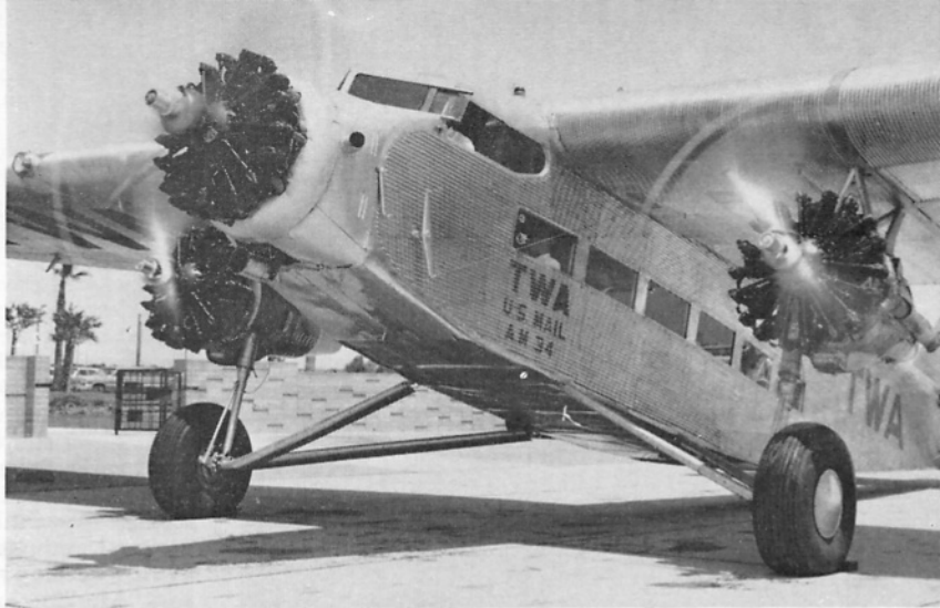
The power and beauty of the Ford Tri-Motor is characterized by this photo of John Louck's 5-AT-C (N414H) taken just prior to its commemorative transcontinental flight in June 1963. Note the BT-13 engines and props and Lockheed 18 wheels.
