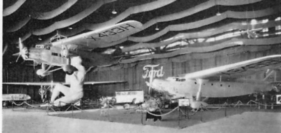
The 1931 Detroit Air Show featured three Fords indoors including the 13-A on the left, and the new single engine 8-AT on the right. The 8-AT is fitted with a Hispano-Suiza in this photo; it was finally delivered to PAA with a Wright Cyclone. (Photo: Ford Archives)
