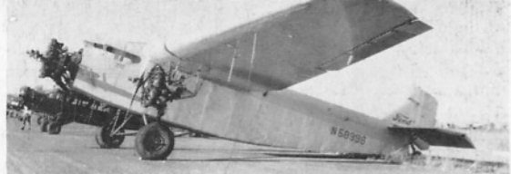
A one-only Ford with "smooth-skin" replacing normal corrugated metal. 5-AT-8 (as XB-NET) was rebuilt in Mexico City in 1951 by Torres Landa; is now owned by Bill Harrah of Reno, Nevada, as N58996. (Photo: L. S. Smalley)
