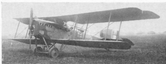
Breguet 14B2 No. 4360 with Liberty 12 engine. This aircraft is remarkable for having the projecting wing portions on the lower wings combined with the late 14B2 wing structure, in which there were no flaps on the lower wings. The revised plan-form of the lower wing tips can be seen and should be compared with that of No. 670 on page 5. As explained in the text, this revised wing arrangement was fitted to Breguet 14B2s that had the horn-balanced ailerons; this aircraft also has wire trailing edges.
