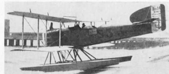
The Bernard float conversion of a Breguet 14B2 of 1924. The twin-float undercarriage could be attached to the normal undercarriage struts of the basic landplane.
