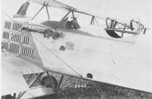
Close-up of cockpits on early Breguet 14A2, probably No. 665. The gun mounting on the rear cockpit is a T.O.A. (Photo: Musée de l'Air 0842)
