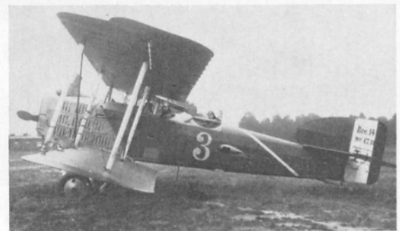
Breguet 14A2 No. 17188 with horn-balanced ailerons and wire trailing edges. Equipped for photographic reconnaissance duties, this aircraft had windshields fitted on the decking between the cockpits.
