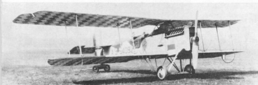
A different Liberty installation in a Breguet 14B2 at McCook Field, U.S.A. This aircraft had the revised 14B2 wing structure with horn-balanced ailerons, together with the later bomb racks that required no forward extensions of the lower-wing leading edges. It bore the U.S. Air Service number A.S.94097 and the McCook Field Project No. P-148.
