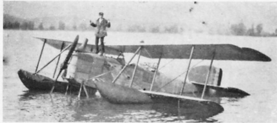
Breguet 14B2 fitted with floatation gear. The aircraft has horn-balanced ailerons, wire trailing edges, the late 14B2 lower wing and underwing skids. (Photos: Jean Noël)
