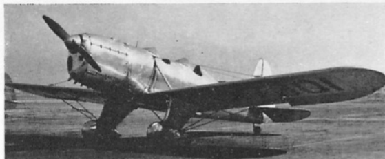
The S-T-A Special, NC17301, powered by a Menasco C-45 engine. (Photo: William T. Larkins)
