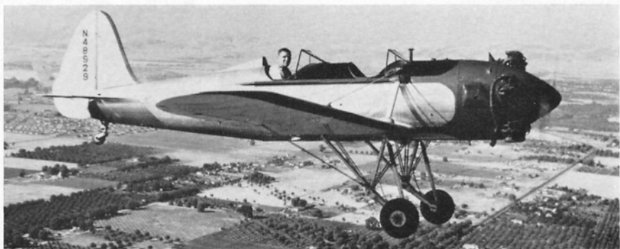
PT-22, N48929, in flight; a cruise at 1,650 r.p.m. and 3,000 feet gives an indicated airspeed of 116 m.p.h. (Photo: William T. Larkins)
