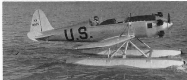
The first S-T-3 converted to S-T-3S configuration with Edo floats. (Photo: Ryan)
