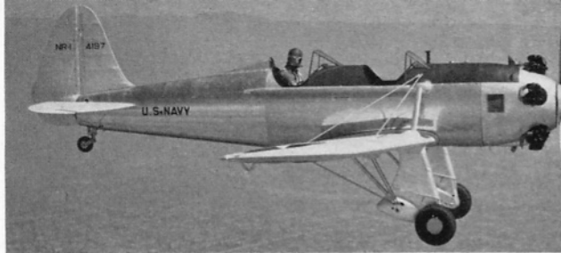
The NR-1 was the Navy equivalent of the PT-21 and the civil S-T-3. (Photo: Ryan via P. M. Bowers)
