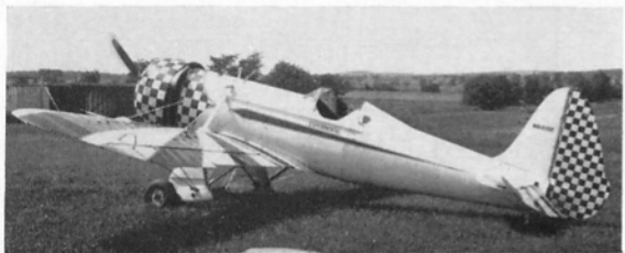
Three converted Ryans: (top) PT-22, c/n 1418 with 220 h.p. Continental engine and Twin Cessna cowling; (middle) a Ranger-powered Ryan of unknown origin; and (below) PT-22, c/n 2056, N60155, with Continental R-670-4 engine.
