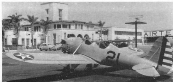
The PT-16A was powered by a Kinner R-440-1 in place of the Menasco L-365-1; the YPT-16's wheel and tail fairings were also removed.
