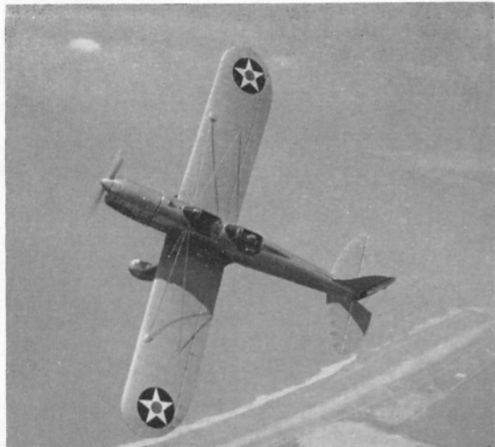
The first XPT-16, 39-717, in aerobatic flight; the PT-16 was the first monoplane trainer type to appear on the U.S. Army Air Corps inventory. (Photo: Ryan)
