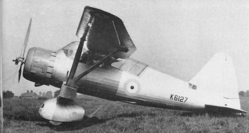
K6127 with stub wings fitted and pilot's step moved aft of mainwheel.
