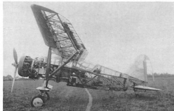
Some intimate Lysander details. Top: The primary fuselage structure (Westland Neg. No. 5660); Second photo: The unclothed second prototype (Ministry of Defence Neg. No. 8925E); Third photo: Close-up of rear cockpit and single Lewis gun mounting (Ministry of Defence Neg. No. 8904T); Bottom: Cockpit layout; notice on extreme left states: "Warning. Bombs on rear carrier: switches Nos. 11, 12, 13, 14 must not be released with message hook down." On the extreme right can be seen the Morse key and a push button marked "Gunner's Attention". (Ministry of Defence Neg. No. 8866)
