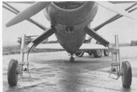
Close-up of the Dowty castoring undercarriage trial installation. (Photo: Westland Aircraft Ltd., Neg. No. 6093)
